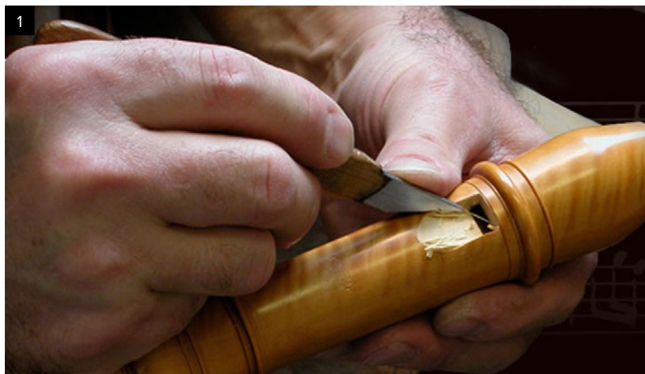
1: Patrick von Huene carving the window of a Denner recorder. (Photo Emily O'Brien)
