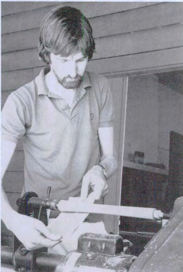
Top right, faculty and students at last summer's San Francisco Early Music Society Instrument Building Seminar. Top left, Alec Loretto demonstrating a technique. Above, Gerry Greer and Joanna Bramel Young measuring and marking tone-hole positions. Left, student Tim Heatn using a lathe to smooth the body of a recorder..
